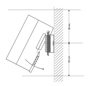
Installed and wired dimensions
